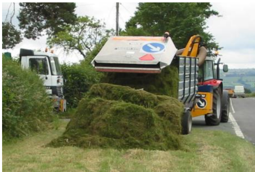
Figure 2.5 A full load emptied from the harvesting machinery at one of the bulking sites
