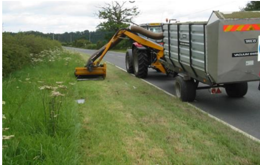
Figure 2.3 Specialised machinery used to harvest vegetation from Powys Road verges
